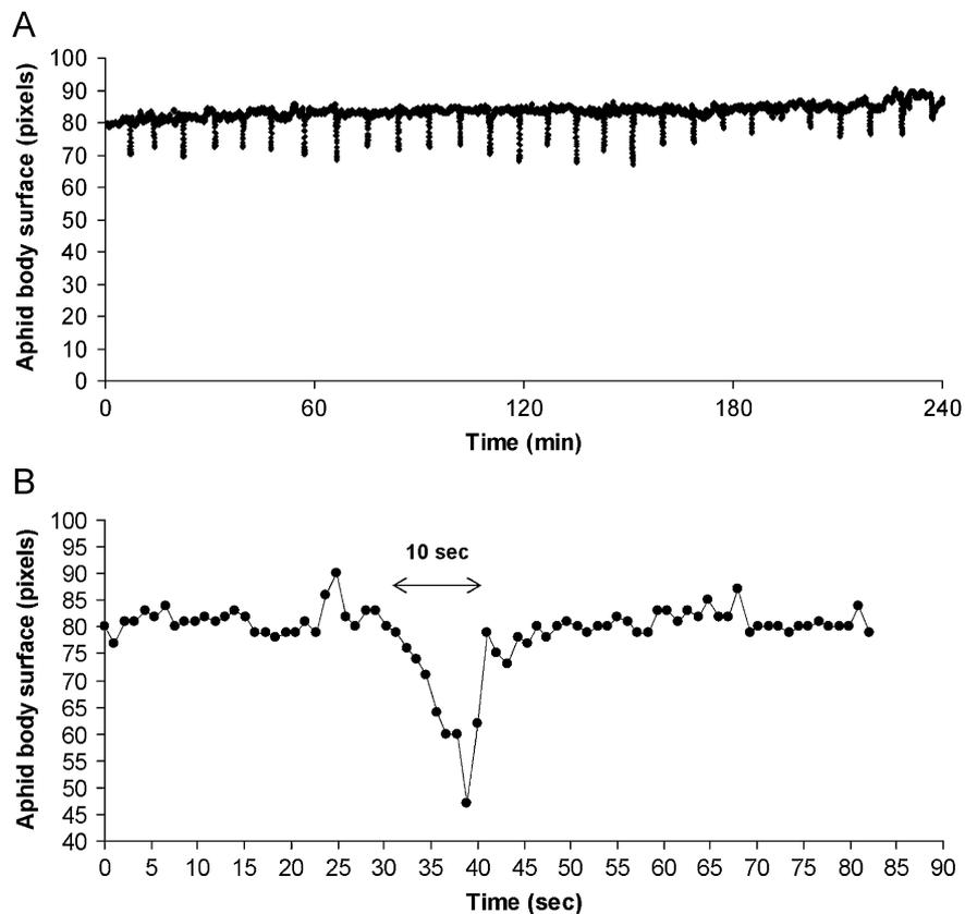
Fig. 2. The body surface of an untreated aphid (in pixels) as recorded by the image analysis programme. (A) Observations over a 4 h period. Brief, apparent reductions in area caused by the lifting of the aphid abdomen recorded as (vertical bars) correspond to honeydew excretion events. (B) A typical excretion event (duration of 10 s); corresponds to the second vertical bar shown in (A).
