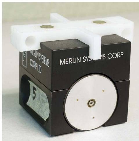
**Fig. 4.** MiaBot Pro wheeled robot with hood and a pair of cylindrical rare-earth magnets press-fit into holes in the hood insert.
